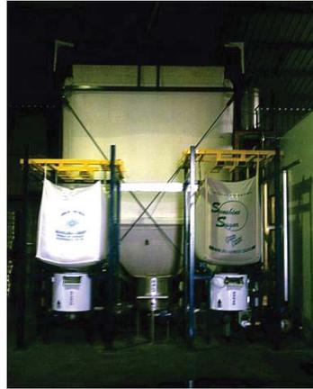
◀ 32t Krause flexible flour silo mounted in 'clean design' frame, (note flour level through walls of silo). This silo is connected to a Krause small ingredient dosing system. It has an "air cone" discharge system.
