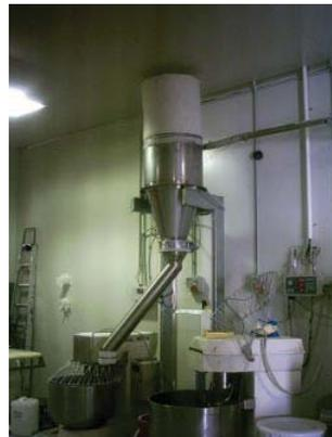
▶ Weigh hopper supported in "free standing" support frame. one of three weigh hoppers connected to a positive blowing system.
