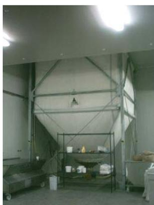
◀ 25t Krause flexible flour silo built to suit available space (rectangular silo) & fitted with vibratory discharger & a positive blowing system.
