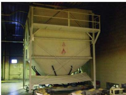
◀ Krause flexible silos and support frames can be fitted with access platforms for easy and totally safe access to the top of the silo for cleaning and maintenance purposes.
