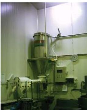
◀ Weigh hopper connected to a vacuum conveying system and fitted with a swivel rotary sifter on hopper outlet.
