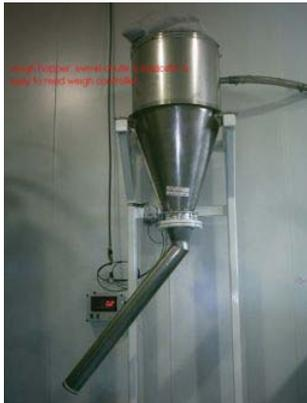
◀ Weigh hopper c/w vent and swivel outlet chute. This hopper is supported on a free standing support frame.
